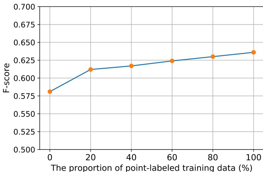
Figure 4.13. SED performance of point models trained on different amount of point-labeled data. The total number of training examples is 6,000. The proportion of point-labeled training data increases by 20% (1,200 examples) from 0 to 100%.
