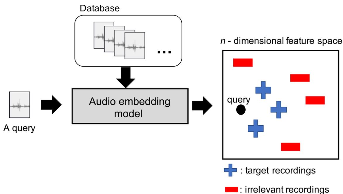
Figure 3.4. An audio embedding model maps recordings into the feature space in a way that similar sound events are grouped together. This makes it easier to find similar sound events to a query using a simple distance or similarity measure such as euclidean distance or cosine similarity
