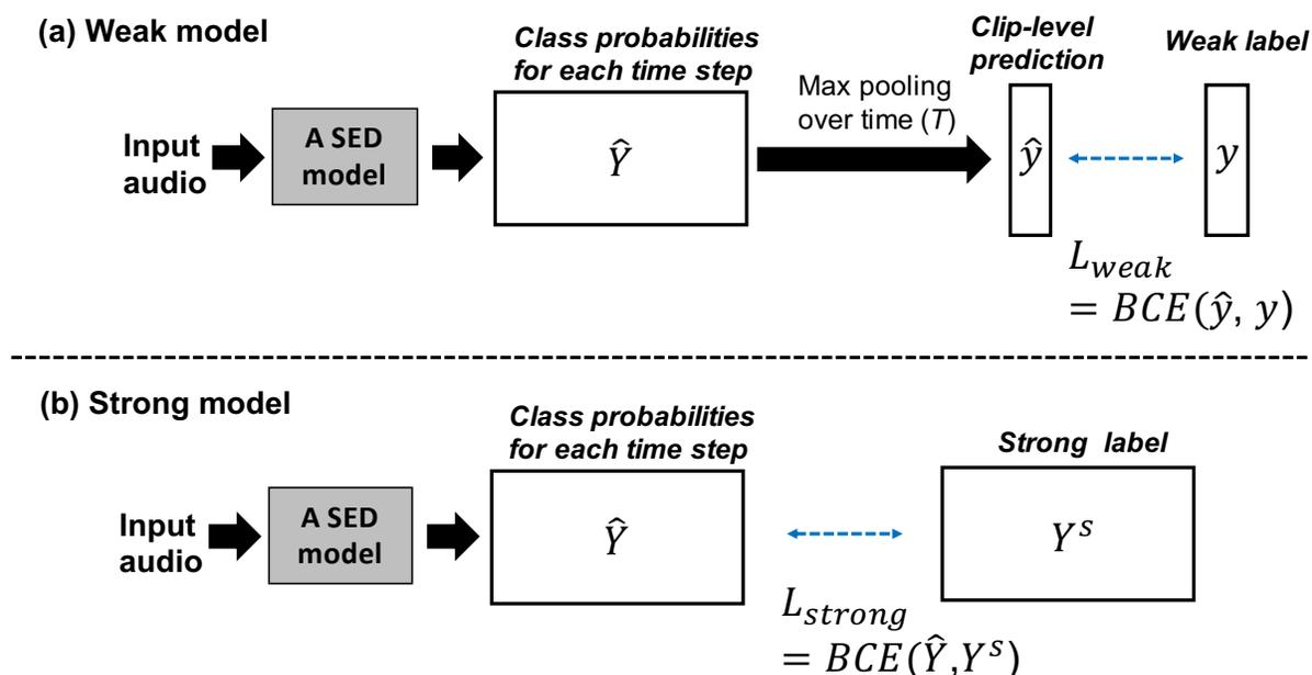
Figure 4.10. Two different ways of computing losses for weak model and strong models. Weak losses  $L_{weak}$  is computed by the difference between clip-level predictions and weak labels. Strong losses  $L_{strong}$  are computed between segment-level predictions and strong labels.
