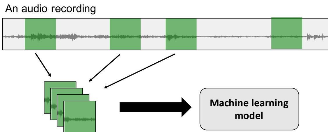
Figure 4.2. For a machine learning model to learn a proper mapping function between an audio signal and its label, each of training examples needs to be well-segmented with correct onset and offset times of an audio event. Therefore, it requires *strong-labels* of sound events in a recording.
