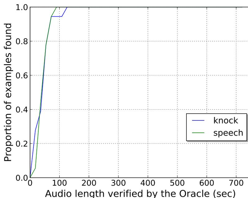
Figure 2.12. The user simulation. The proportion of examples found according to the proportion of audio the oracle evaluated. All sound events are detected by evaluating less than 126 seconds of the audio (17.5% of the audio).
