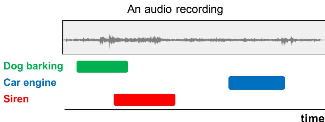
Figure 4.1. Examples of Sound Event Detection (SED). Given an audio recording and a fixed set of sound classes, a SED system automatically identifies the classes of sound events and estimate temporal locations (i.e. start and end) of the events within the recording. There could be multiple sound classes overlapping each other (i.e., polyphonic environment)
