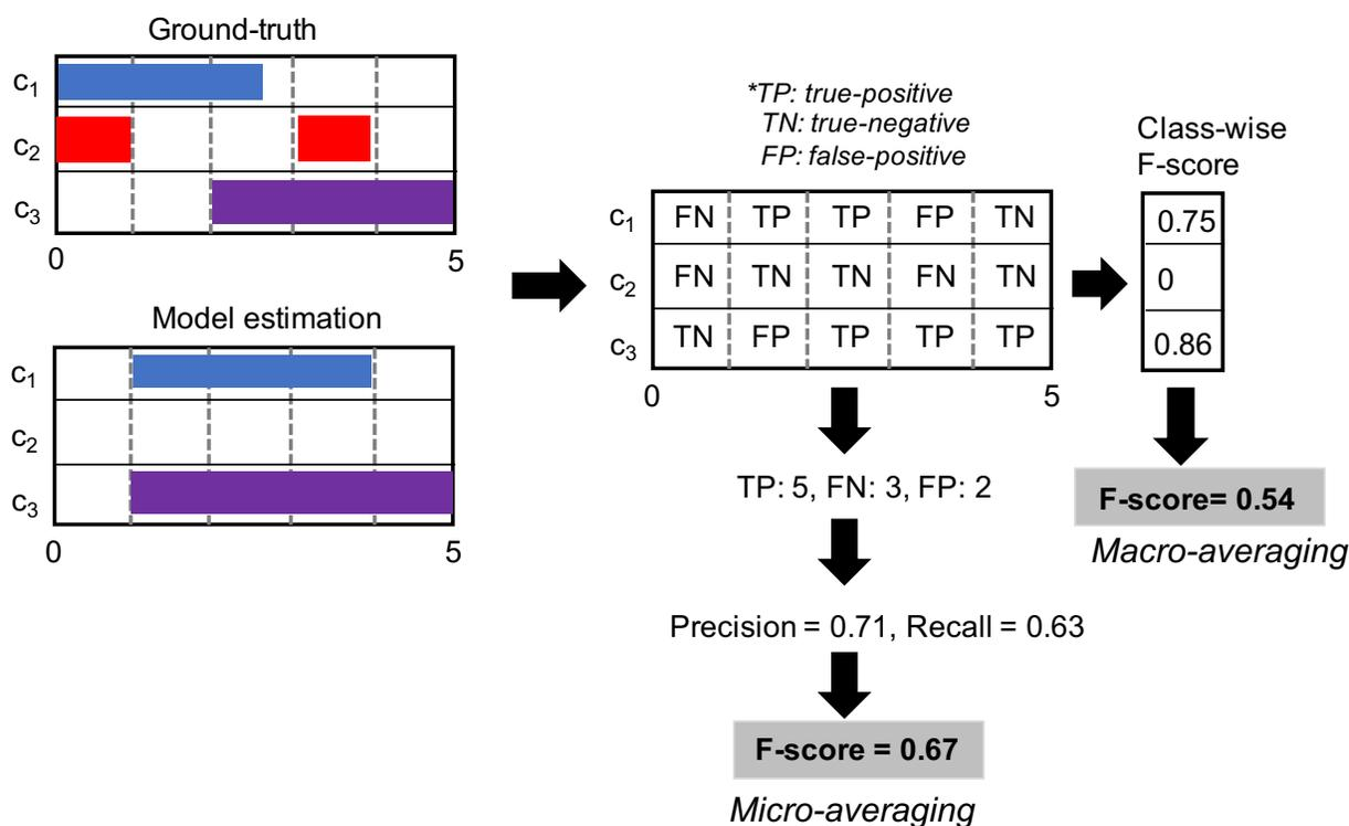
Figure 4.7. An example of computing segment-based  $F_1$  scores with micro and macro averaging on a 5-second audio clip.
