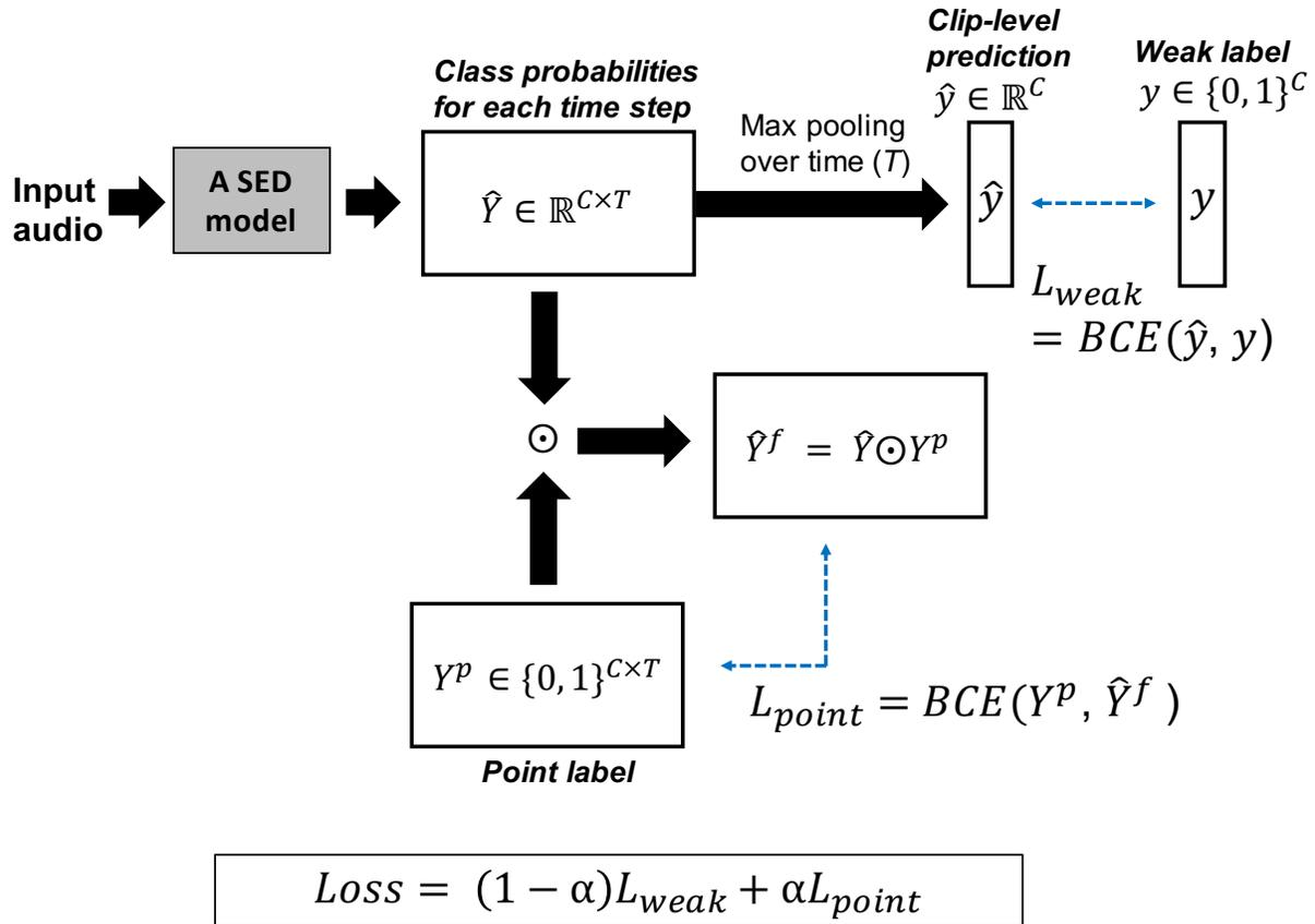
Figure 4.5. Summary of computing losses on point-labeled audio data during model training. It is trained to minimize the combination of weak loss and point-label loss. \*BCE refers to Binary-Cross Entropy loss
