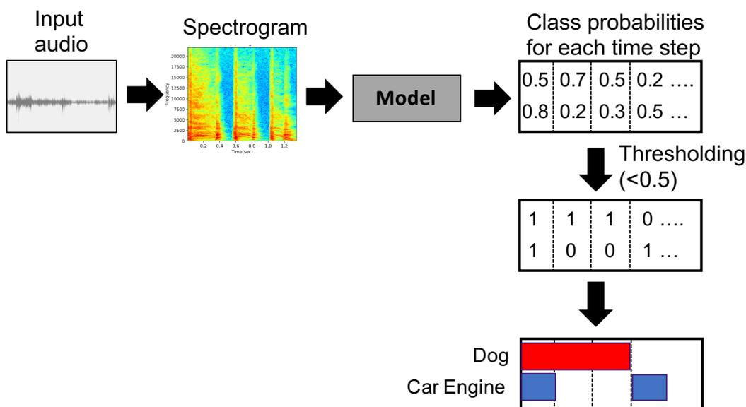
Figure 4.8. An example of how a trained model performs sound event detection given a test audio clip
