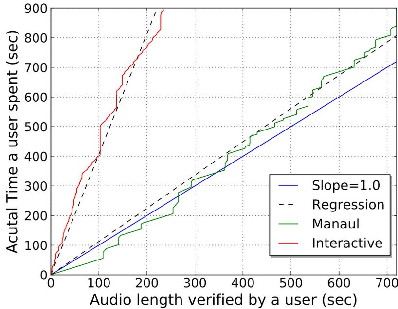
Figure 2.10. Total time a participant (one participant is selected as an example) spent on the task as a function of the total amount of audio verified/labeled. The interactive system requires more time to label a fixed amount of audio than the manual system. This interaction overhead partially offsets the speedup of the overall task the interactive system provides by having the users label the most promising segments of audio first.
