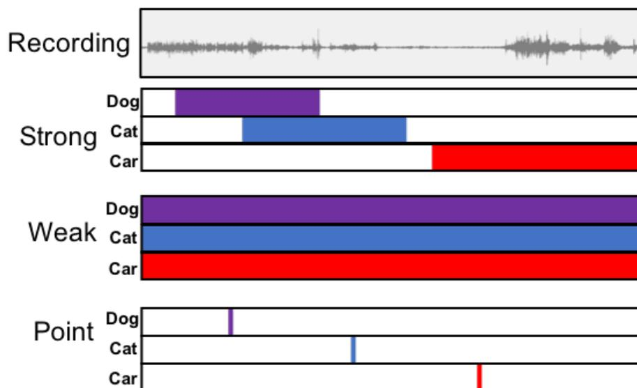
Figure 4.3. Examples of different types of audio annotation. Strong labels contain names of sound events and their time information. Weak labels only have clip-level presence or absence of events without their timing information. Point labels contain names of sound events at a single time point per sound event instance within a recording. The position of each point can vary within each instance.
