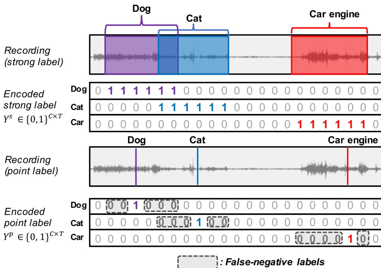
Figure 4.4. Examples of how to encode point labels to compute point-label loss. In this example, three sound events are present at different time location within an audio clip, which result in three point labels at three different time positions. It also illustrates false-negative labels generated by the encoded point labels.
