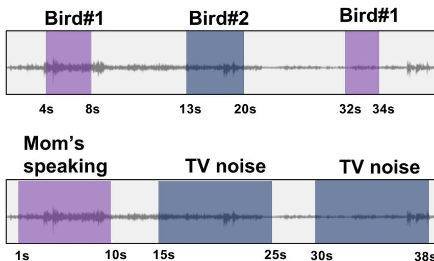
Figure 1.1. Examples of sound event annotation. Each sound event of interest is labeled with a text tag and its temporal location within a recording.
