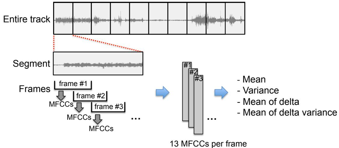
Figure 2.2. Audio feature extraction for all segments of an audio file. MFCCs are extracted frame-wise and pooled over each segment using the means and variances of both the instantaneous and delta values.
