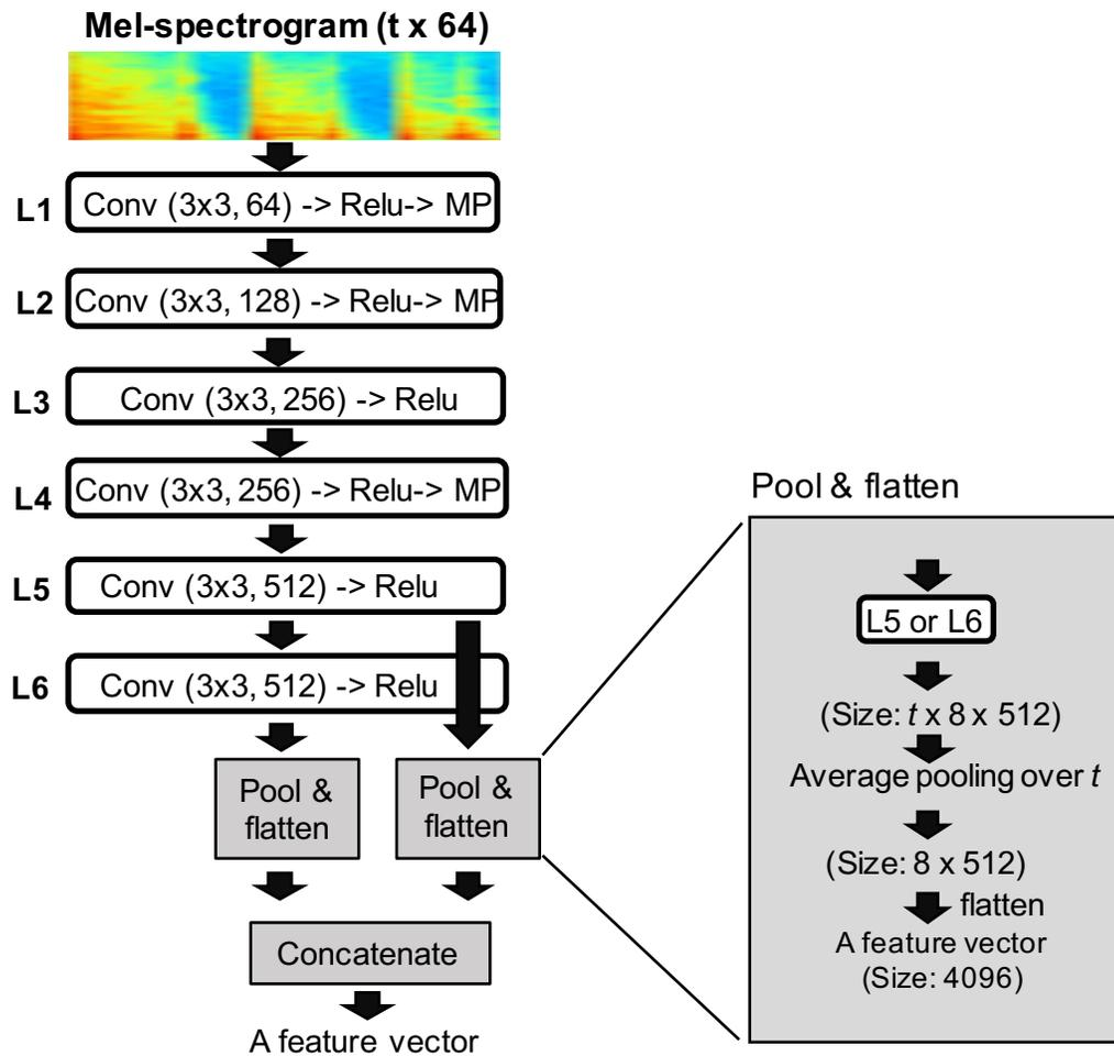
Figure 3.6. The proposed CNN-based feature extractor. The information for each filter is denoted as (width  $\times$  height, channels) in each layer block. MP indicates max pooling operation. ReLU activation functions are used for every convolutional layer. Outputs from layer 5 and 6 are concatenated to build a single feature vector
