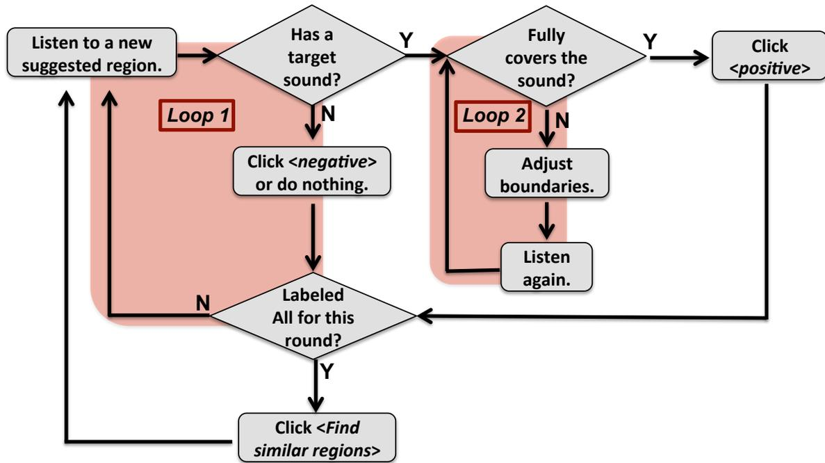
Figure 2.14. There are two bottlenecks (Loop 1 and Loop 2) in the interaction flowchart of the interactive annotation.
