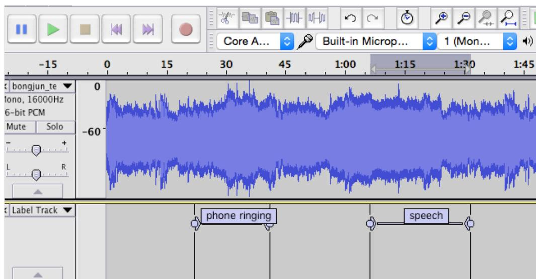
Figure 1.3. An example of sound event annotation tools: Audacity [64]. A user can load a label track in addition to an audio track and add a text tag with its temporal locations (onset and offset of a sound event).
