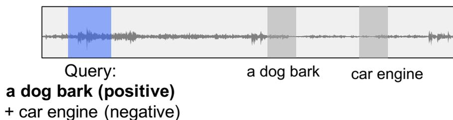
Figure 3.1. An example of the problem on a query containing overlapping sound events. Given such a query, the retrieval system does not know which portion of the query is relevant to a sound event that a user wants to search.
